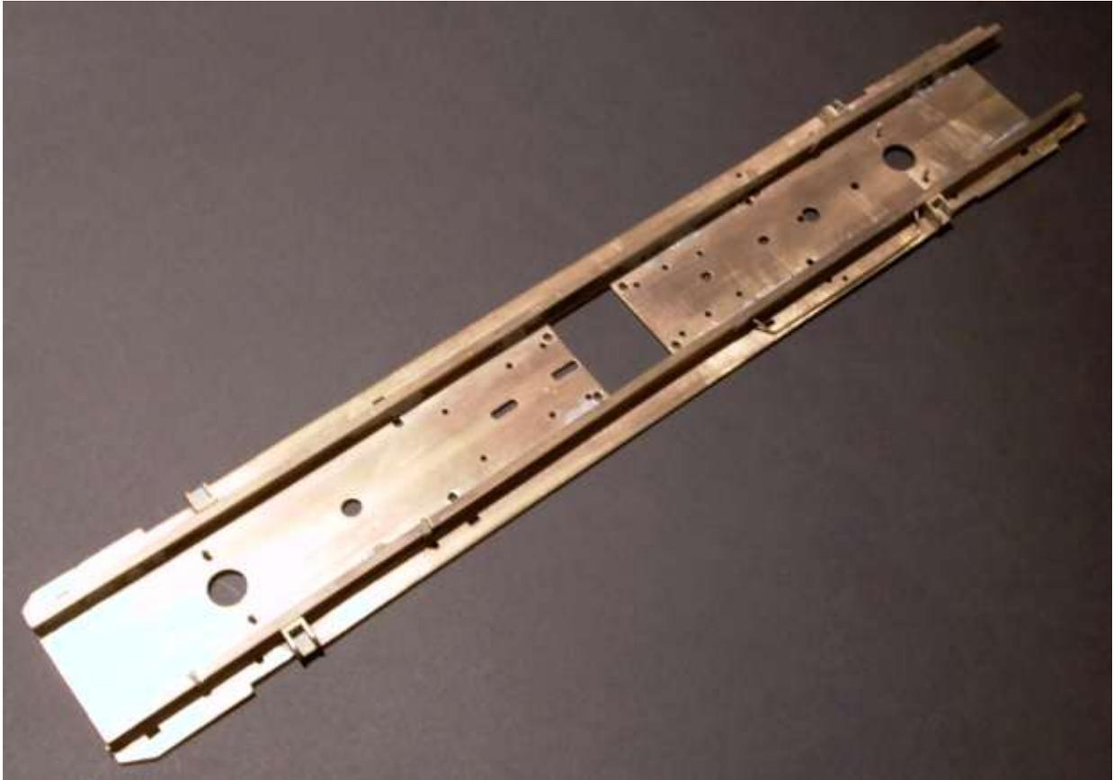
A little bit of rosin, some electronic solder, my precious torch from Home Depot, and the rails, pipes and hoses were placed back on the main plate and soldered with some fat and healthy mix of tin and silver. And, great news, this time the chassis was flat (Turbine-03). The rosin was cleaned with alcohol, and the parts and excess of solder were nicely sanded and filed.
