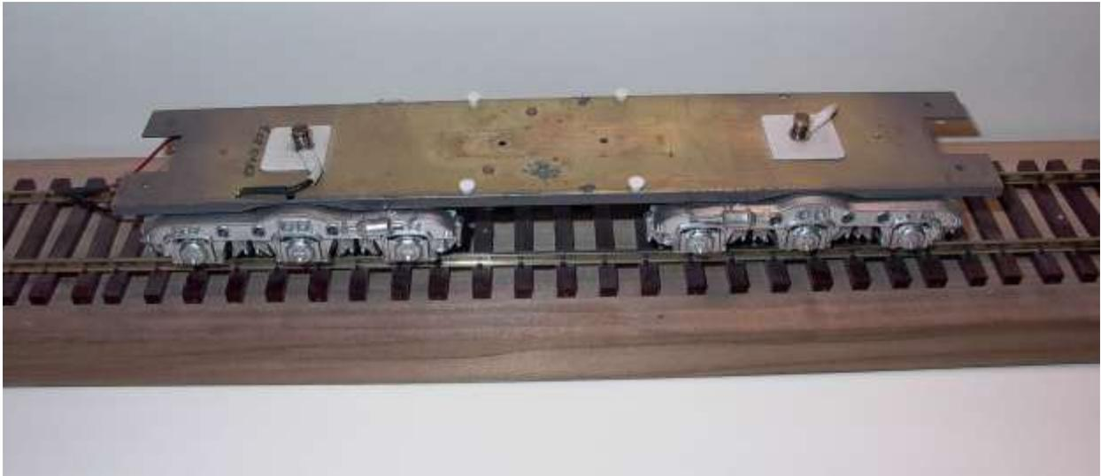
The original springs and bolts are used to install two wires leading to the common power bus. The most difficult part was to route the wires underneath the tender chassis so as to not obstruct or disturb the rotation of the trucks. The top of the tender was not an option to route the wires as the shell has some stiffeners that are sitting flush on the chassis of the tender (Tender-03).
