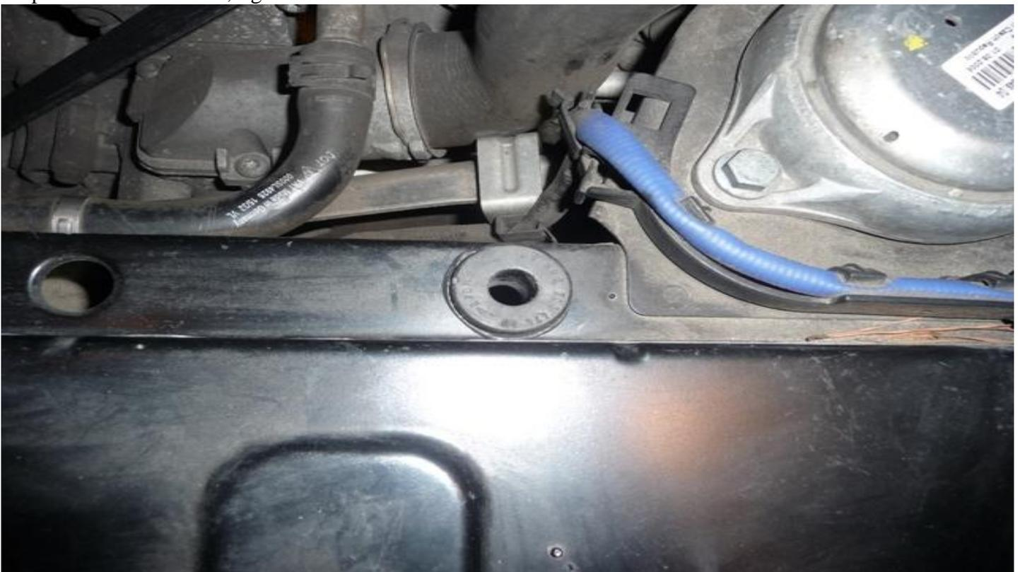
4) The engine compartment is now open. Tuck gently the two electrical wires and the vacuum line on the side:
