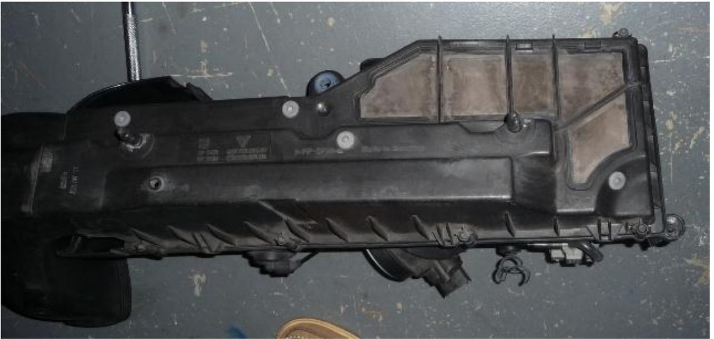
6) The air filter box can be opened with your T25 TORX screw driver. There are 8 screws to be unlocked all the way (do not remove them from the box). The filter element is easily swapped with a new one. I usually write mileage and date on the side of the filter element with a Sharpie.
