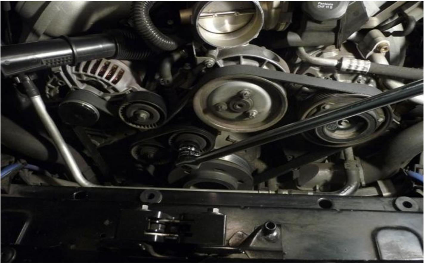
Now, using your hand, gently push on the break bar (clockwise) to move the belt tensioner closer to the pulley. Do not be afraid to push, as the hydraulic spring is quite strong.
