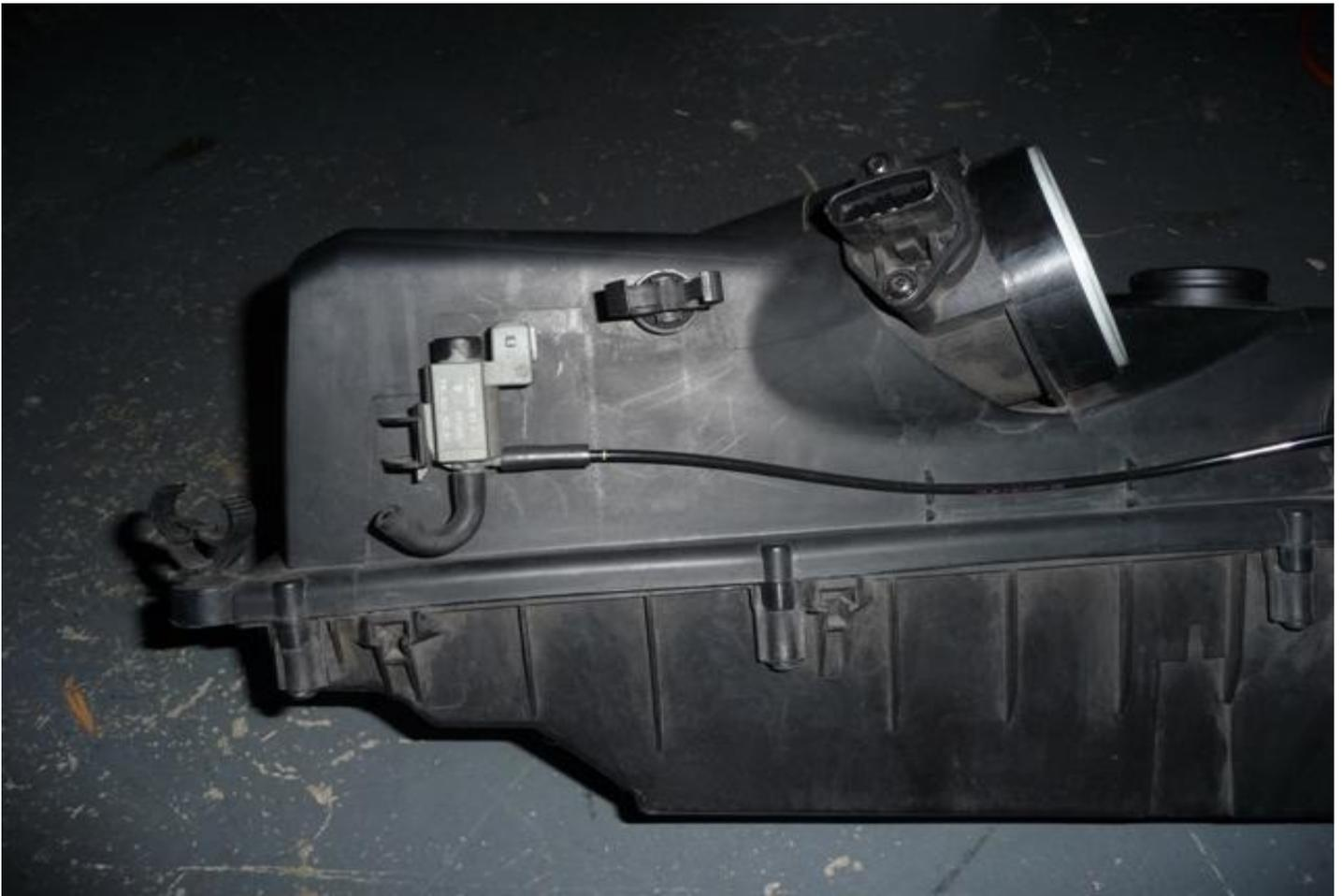
3) The filter box holds only thanks to three prongs (two underneath and one on the rear). When pulling and wiggling the box out, be very careful as to not lose the two rubber grommets located at the bottom of the box. To prevent such accident, I glued mine to the frame:
